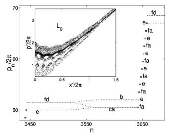
FIG. 4. Magnification of one step in the chaotic flight shown in Fig. 3. The horizontal part of the step (dots) consists of *efd* cycles followed by *cab* cycles (total of 198 points). The vertical part (squares) consists of six acceleration cycles *fae* (18 points). The inset shows the acceleration spot  $\{a(L_0)\}$  in unit cell j=0 using the variables  $x' = (x + \pi) \times 10^5$  and  $p' = (p + \pi) \times 10^5$ .
